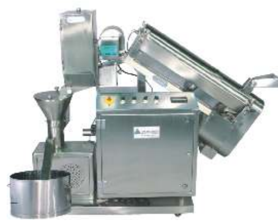
Capsule Polishing Unit with Filled Capsule Sorter and Unfilled Capsule Separator
